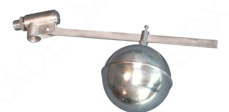
Size : DN3/4" Connection : Male BSP Min Temperature : -5°C Max Temperature : +90°C Max Pressure : 8 Bars (6 bars for ball D.180) Specifications : Settable compensator Horizontal position Stainless steel valve
